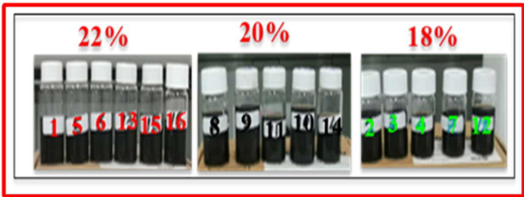
Figure 1: The Prepared samples of CNAs with three ratios of Al 2 O 3 at different conditions.
