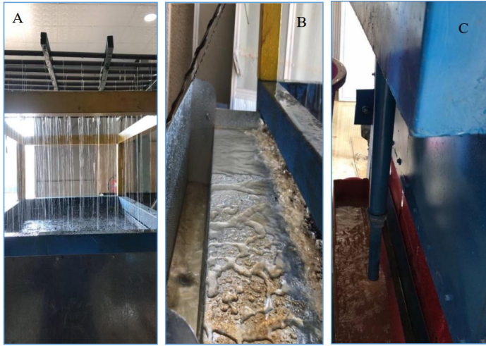
Figure 2: The collected runoff water under pavement layers A) Rainfall simulator system; B and C) Surface and Subsurface runoff.
