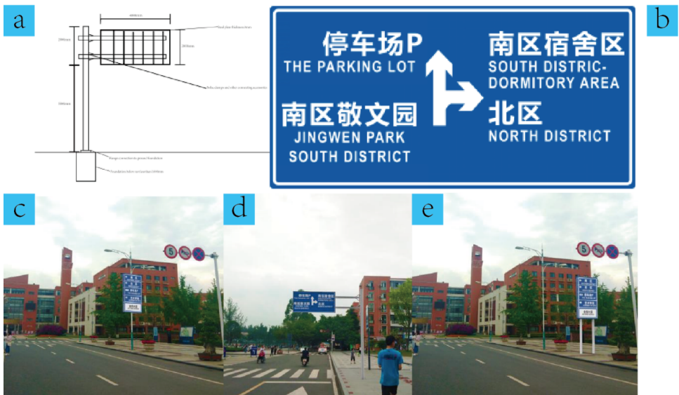
Figure 16: (a) How to install a car navigation sign, (b) Design specifications for vehicular guide signs, (c) Effect of secondary vehicular guide signs combined with street lighting, (d) Effect of primary guide signs, and (e) Effect of secondary guide signs.
