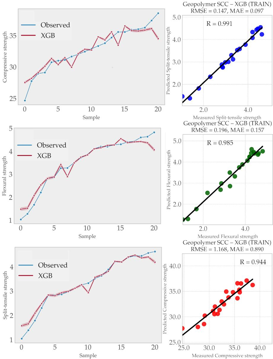
**Figure 5:** Left: Comparison of observed and predicted values averaged (over 30 runs). Top: Compressive strength, middle: Flexural strength and bottom: Split-test strength. Right: Scatter plots for the best model in 30 runs according to RMSE for Compressive strength, Flexural strength and Split-test strength.
