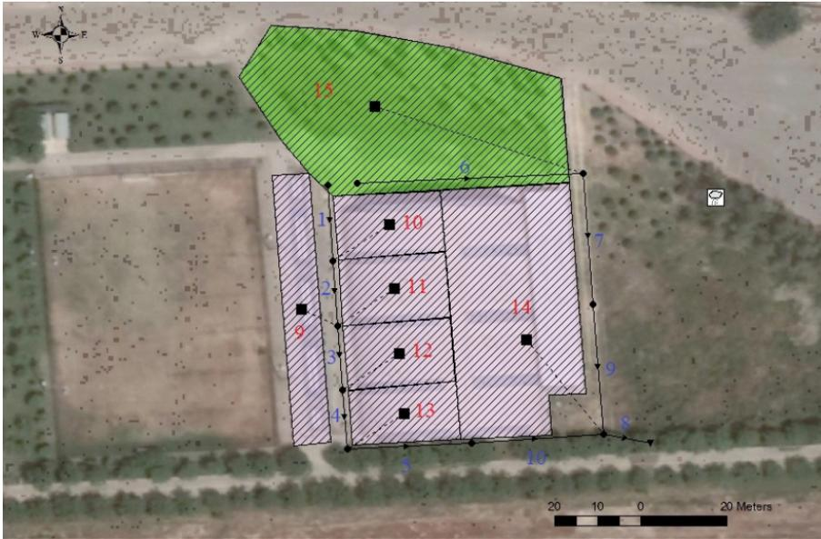
**Figure 9:** Model Sub-catchments and drainage lines.
