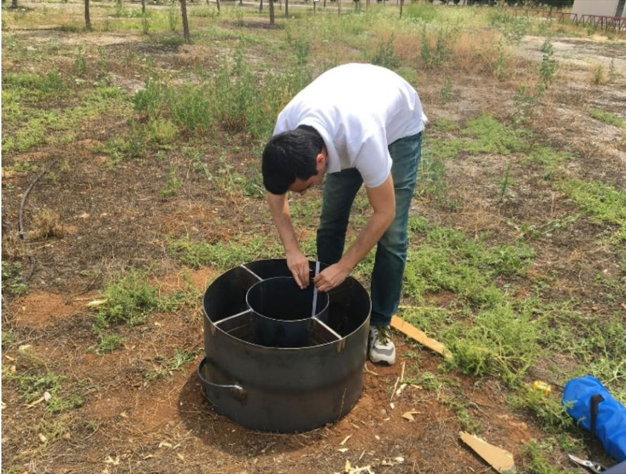
**Figure 5:** Double ring infiltrometer setup at the study area.
