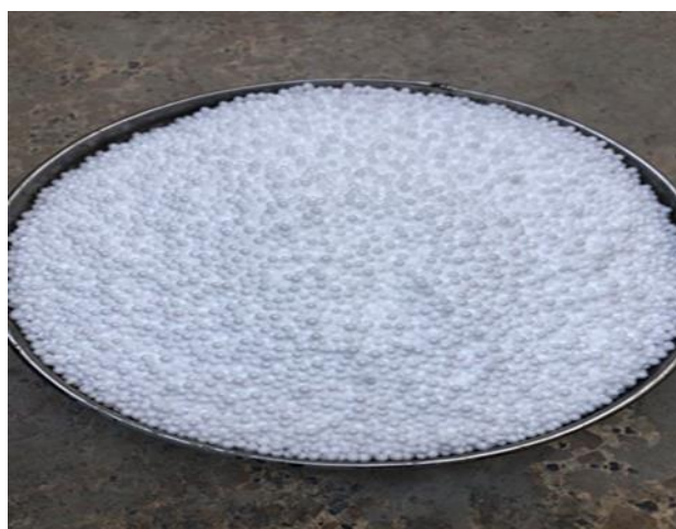
Figure 4. Expanded polystyrene beads (EPS) used in the experiment.
