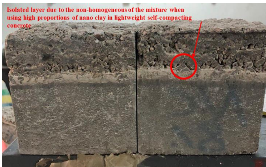
Figure 6. Clarifies concrete cubes with a ratio of 8% NC.
