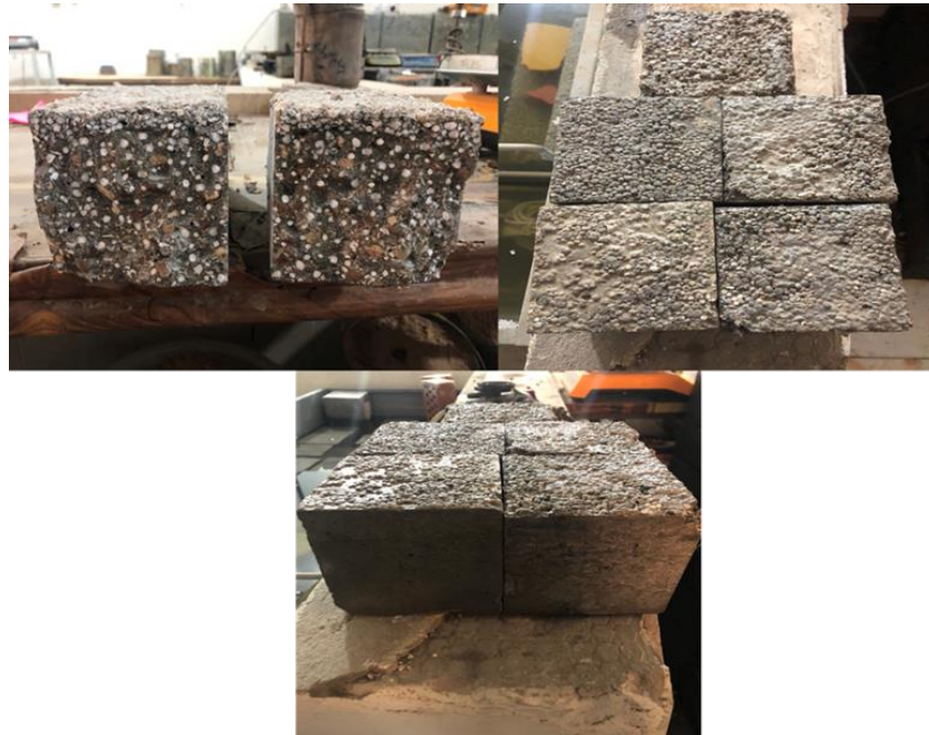
Figure 8. EPS distribution pattern in concrete specimen.
